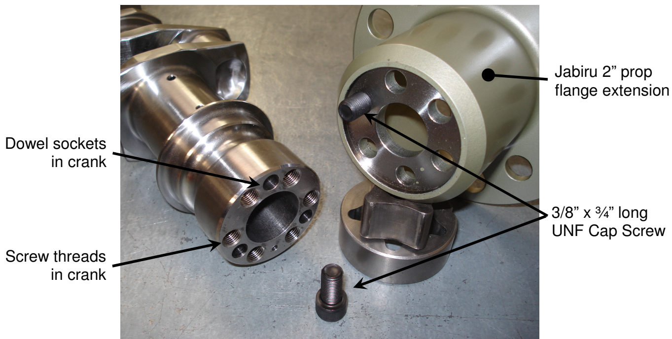
Figure 1 – Flange & Crankshaft
