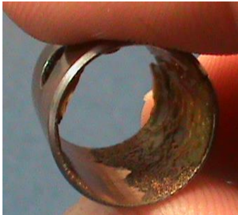
Figure 3: Badly worn rocker bush.
